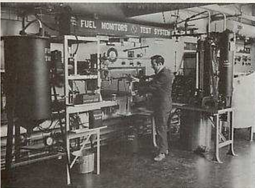
Fuel cleanliness system components are evaluated with a contaminated fuel supply.
